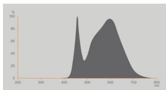
EPREL Data Spectral Diagram LEDr
