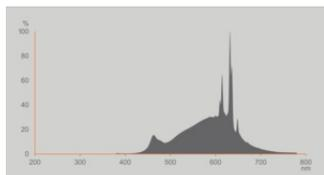
EPREL Data Spectral Diagram LEDr
