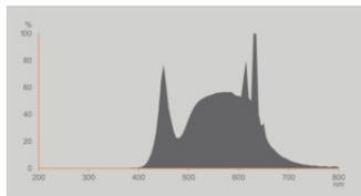
EPREL Data Spectral Diagram LEDr
