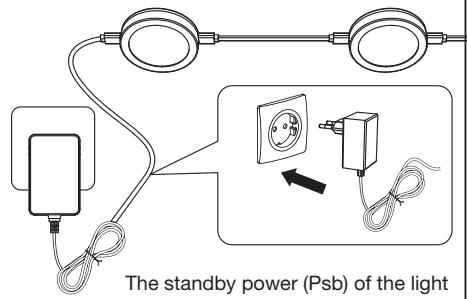
The standby power ( $P_{sb}$ ) of the light source is less than 0.5W.\*\*\*
